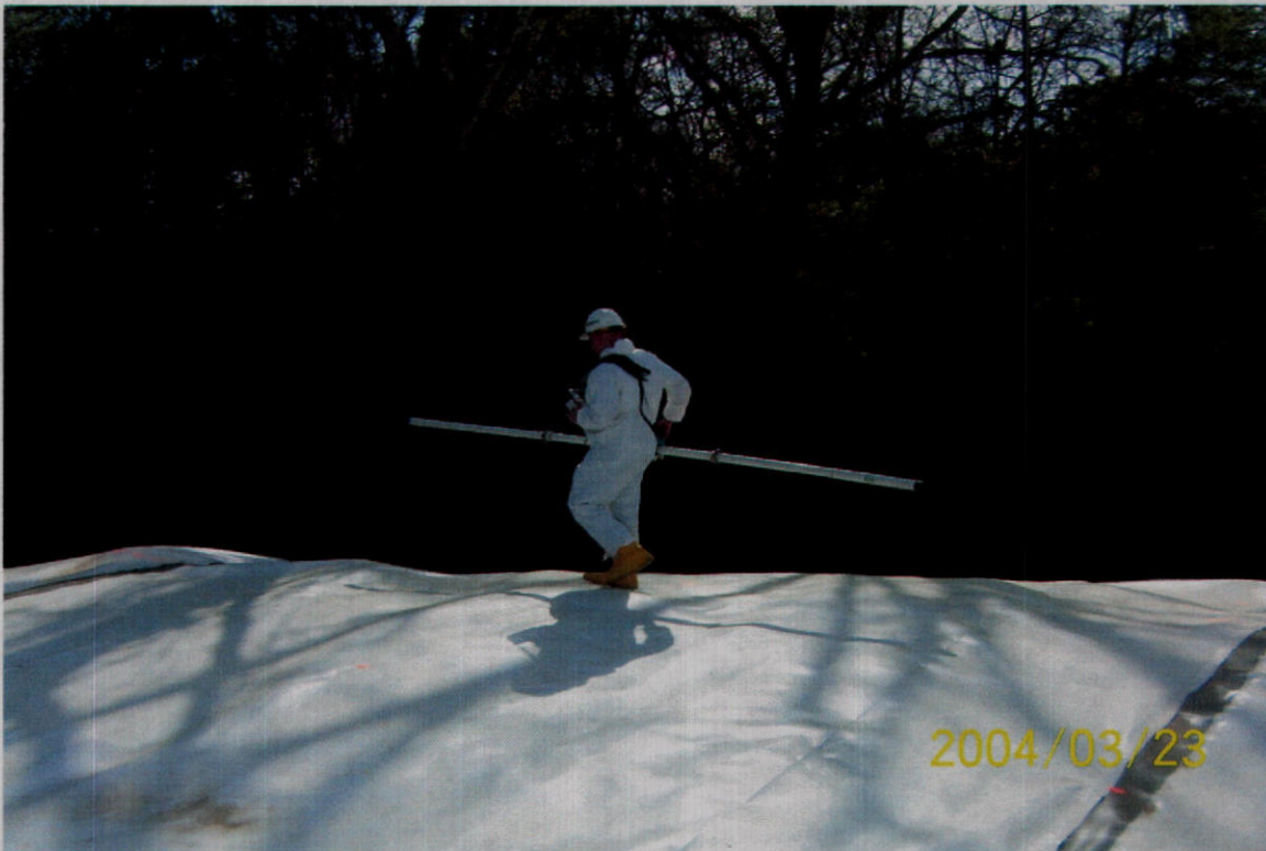
PHOTO 4 – View of the Schnabel Engineering project manager gathering data for the electromagnetic (EM) study portion of the geophysical survey. The EM study was conducted to identify areas containing metallic debris.
